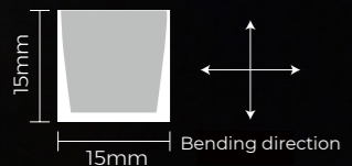
Creative design for various applications of top bend and side bend in 3D space
